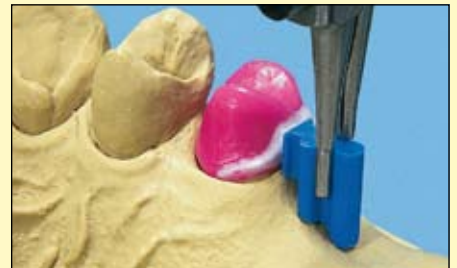
Placing the attachment, scraping wax surfaces parallel or conical – all this can be done with the BF 2.
