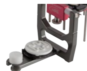
Place Connect mounting plate in the articulator.
