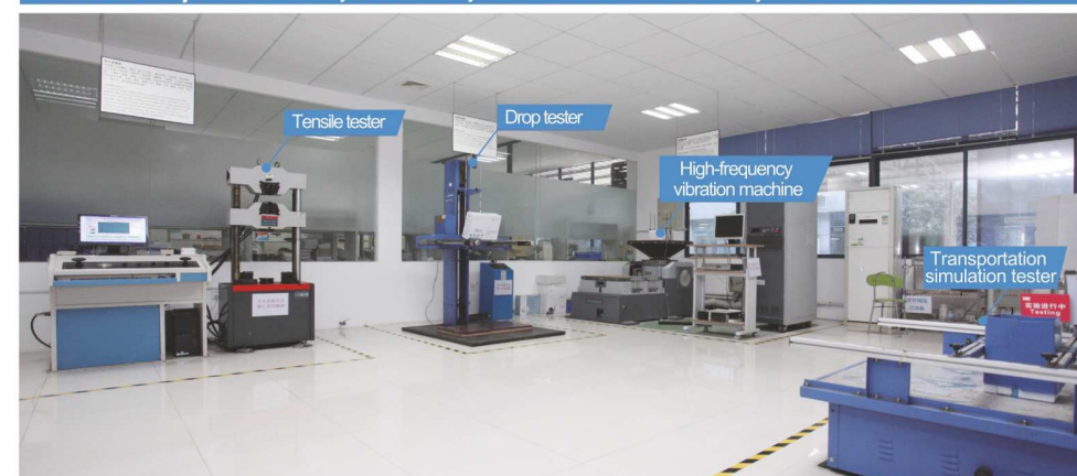
Mechanical environmental laboratory Simulate various extreme mechanical environments to ensure high-quality of products.
