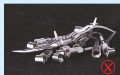
Tips of poor quality start to be cracked after one-hour working, the cracking rate within 10 hours is 35%.
