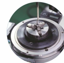
Roundness measuring instrument Japan-imported, high degree of accuracy(0.01um)
