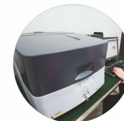
Energy dispersive X-ray fluorescence spectrometer To detect the harmful material, keeping with the demand of EU standard
