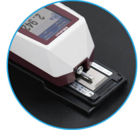
Roughness detector Japan-imported, to test the roughness of metal surface
