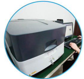
Energy dispersive X-ray fluorescence spectrometer To detect the harmful material, keeping with the demand of EU standard
